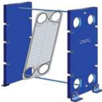
1. The frame is put together. It consists of frame and pressure plates, top and bottom carrying bars and connections. The end plate is the first plate to be hung in the frame.
