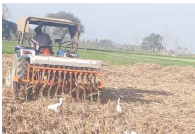
RDD used for sowing of wheat in full residue load in sugarcane ratoon and wheat crop in sugarcane residue
