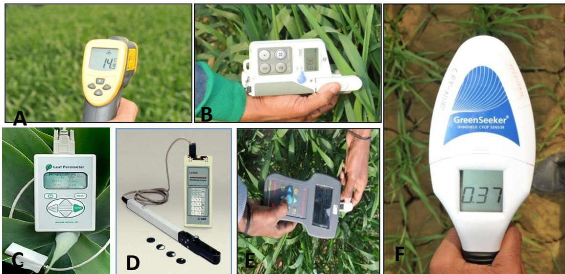
Fig.1: Different physiological instruments used in field phenotyping (A) Infra red gun (B) Chlorophyll meter (C) Porometer (D) LAI meter (E) CFL meter (F) NDVI
