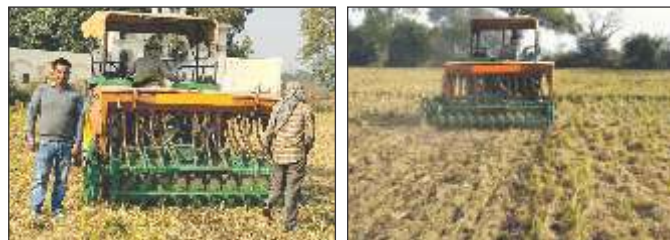
Fig. 4.10. Field demonstrations of Smart Seeder (Strip-till Drill) for direct sowing of wheat in rice residue
